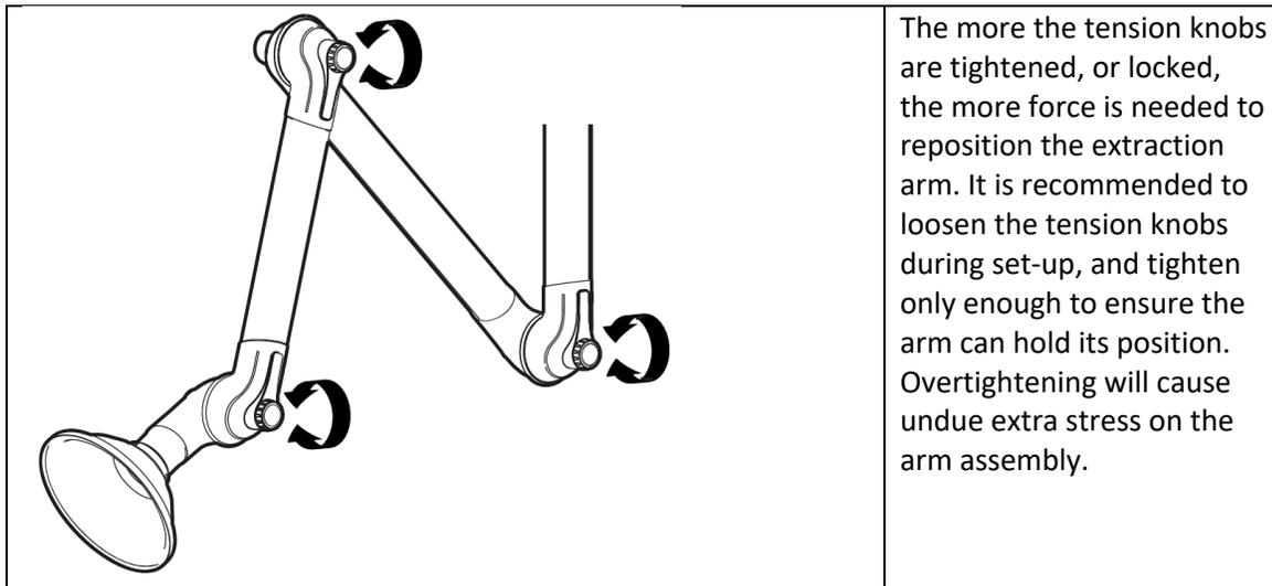
To move arms in position and ready for use, the tension knob (lock) needs to be loosened to allow arms to move freely. If the tension knobs remain in locked position, the stress on the arm can cause damage to the friction joints, hood assembly, and gas-shocks.
